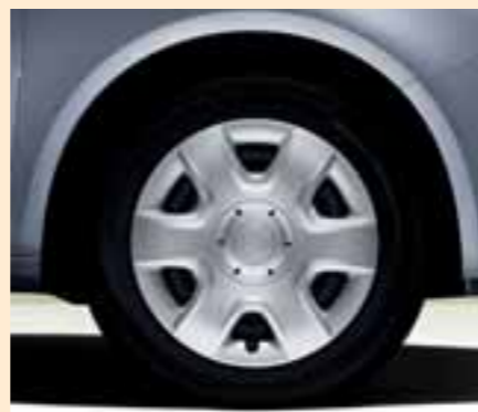
6.0J x 15" steel wheels for 195/55 R15 tyres with Hermes hub covers.
